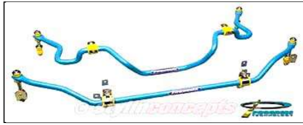
Fig.2 - Sample anti-roll bar geometries
