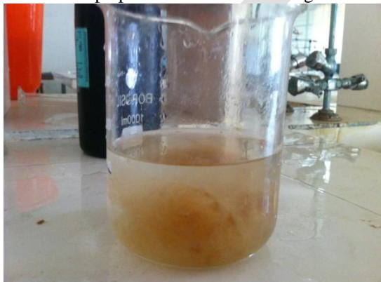
Fig.18:soda pulp after bleaching
