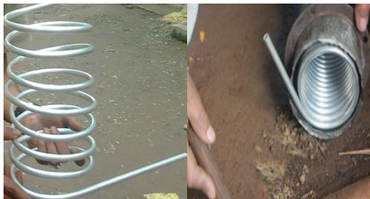
Fabricating first Prototype (Aluminum Coil Inside)
