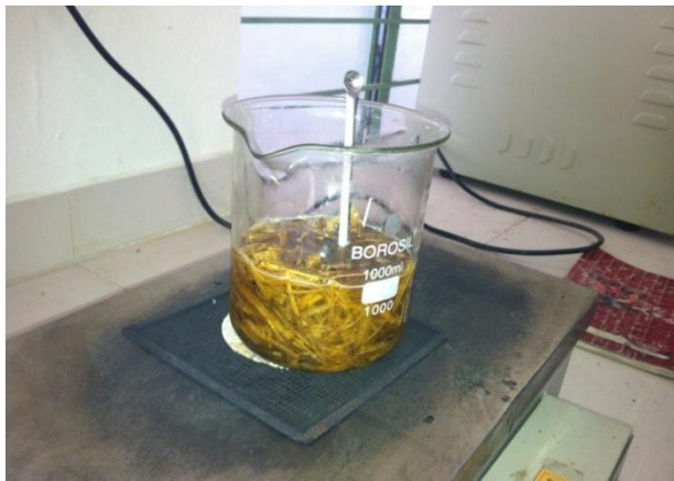
Fig.10: cooking liquor and raw material
