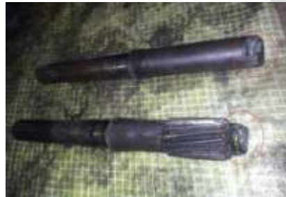
Fig.1 .failure of shaft
