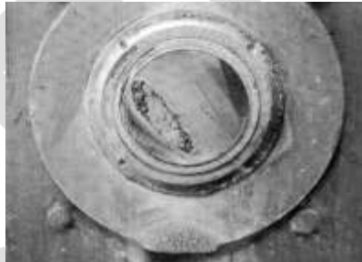
Fig.2. Failure caused by rotational bending [3]
