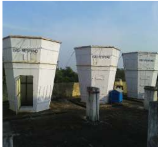
FIG 7: SODAR antenna at Dept. of Systems Design, Andhra University. Sponsored by UGC and ISRO.
