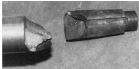
Fig. 4. Failure due to reverse torsional loading [3]
