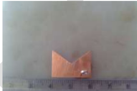
Fig 2 Manufactured rectangular microstrip patch antenna
