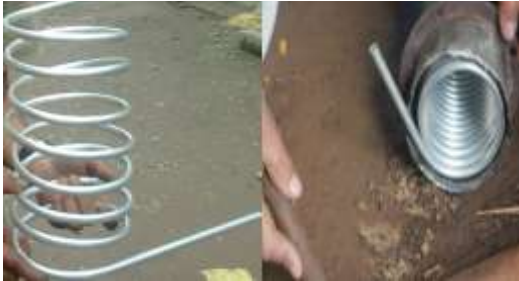
Fabricating first Prototype (Aluminum Coil Inside)
