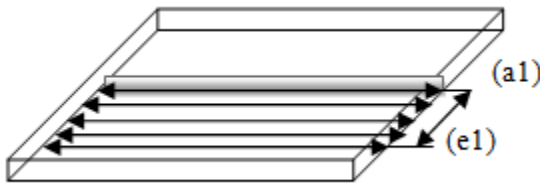
Fig.18.Distortion along different longitudinal lines parallel to weld
